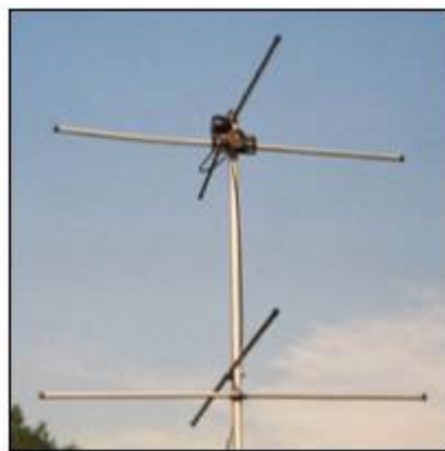
Figure IV-2 Omnidirectional "turnstile" Type Antenna for APT Reception
