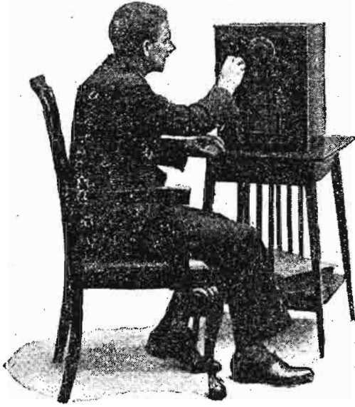
Fig. 1.—The set is housed in a cabinet constructed on modern lines, including a sliding frame, space for speaker, batteries and accumulator.
