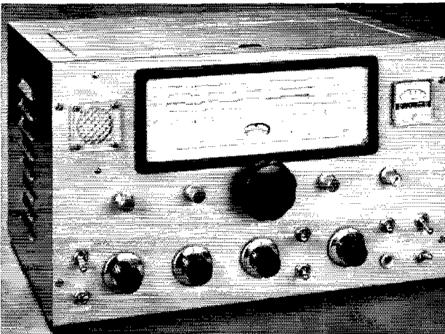
The HBR-13C, built by Alexander Stewart, WA4ZNI, is the basic HBR-11 or HBR-12 plus the additions and modifications described in the text. Major electrical changes are the addition of an amplifier stage at the first intermediate frequency (1610 kc.) and one more transformer in the 100-kc. second-i.f. amplifier. The mechanical arrangement permits centering the large Eddystone dial.
