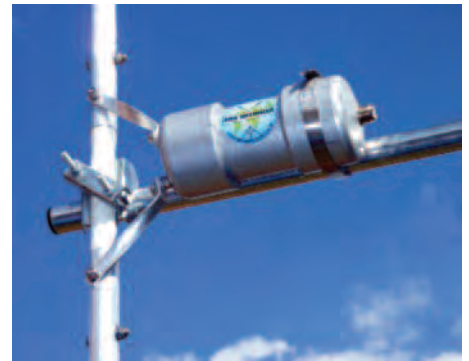
A close up of the un-un at the feed point.
